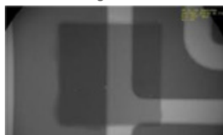
Solder joint made using the vacuum module (vacuum range: 5 Torr / 30 sec.)
